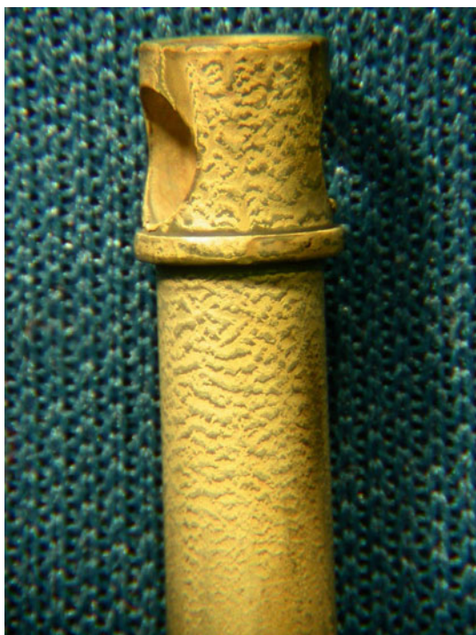
Fig. 10 Surface of an Ag-Sn alloy coating deposited from electrolyte 3 on a contact pin at 14 \text{ mA dm}^{-2}
